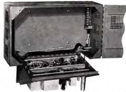
Figure 7 — 12A Power Unit. View shows equipment swung down to expose wiring.
