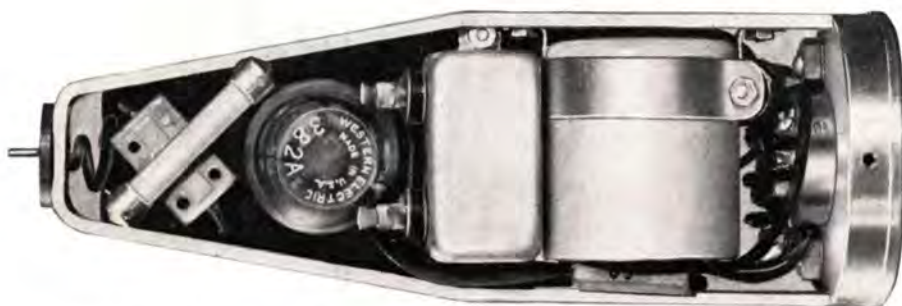
Figure 11 — RA-1095 Amplifier with Cover Removed.
