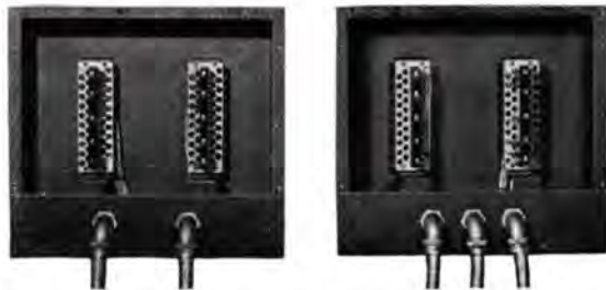
Figure 8 — 7A Junction Box (left) and 7B Junction Box (right) with cover plates removed.
