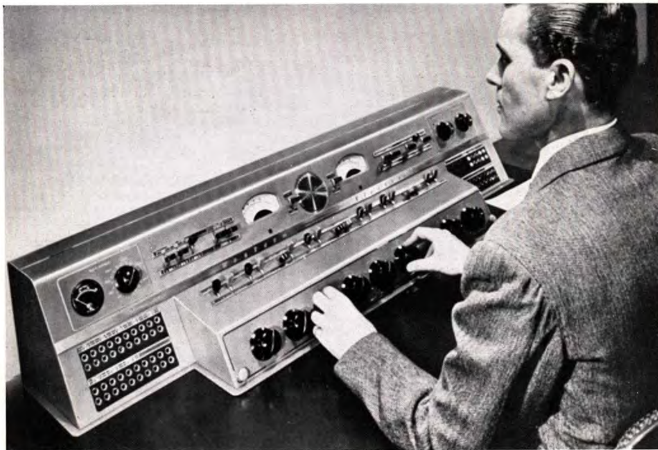
Figure 4—Operator at 40A Console of 25B Speech Input Equipment. Controls are grouped functionally with frequently used controls nearest operator and all controls within convenient reach.
