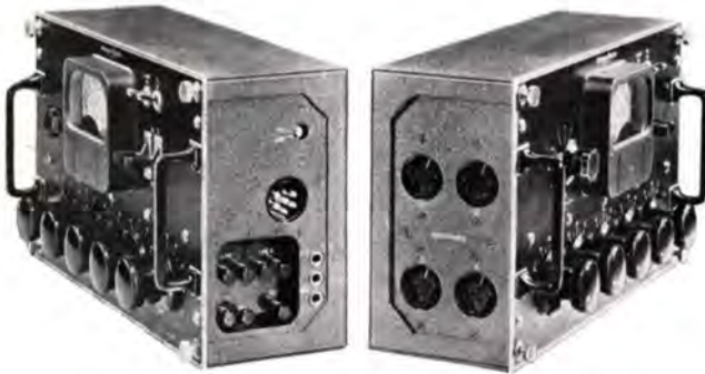
Figure 21 — Left: Right end of the Amplifier-control Unit showing line terminals, telephone binding posts and plug, plug for monitoring headset and the multi-pronged socket for the power supply plug. Right: Left end of the Amplifier-control Unit showing four plug-in type microphone receptacles.
