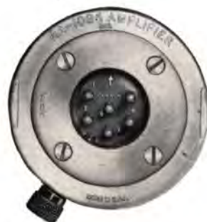
Figure 12 — Base of Amplifier Showing 6 Prong Socket.
