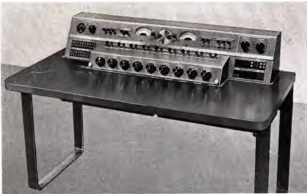
Figure 5 — 40A Console mounted in KS-10284 table.
