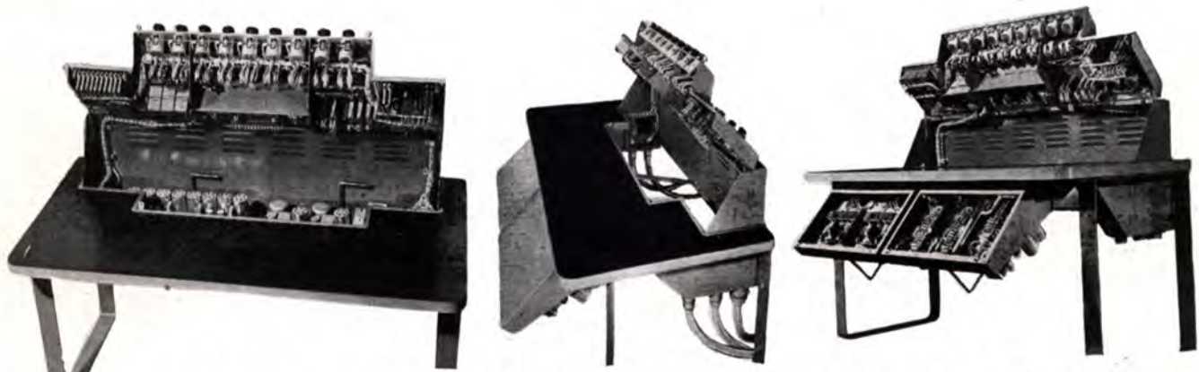
Figure 6 — Three views of the 25B showing the 40A Console and the KS-10284 table with control panel raised and amplifier racks lowered. View at left shows the control panel lifted for access to all keys, jacks, potentiometers and control apparatus and wiring in 40A Console. Lifting this panel also exposes tube side of all amplifiers. Center photo-
